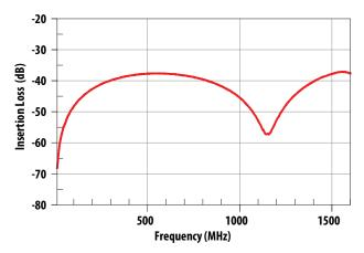
Figure 9. Tx–Ant Low Frequency Rejection.
