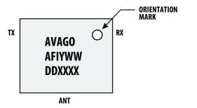
Figure 29. Product Marking and Pin Orientation.
