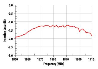
Figure 1. Tx–Ant Insertion Loss.
