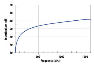
Figure 10. Ant–Rx Low Frequency Rejection.
