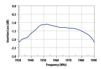
Figure 2. Ant–Rx Insertion Loss.
