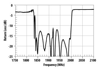
Figure 6. Antenna Port Return Loss.
