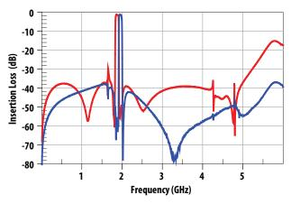
Figure 7. Tx–Ant and Ant–Rx Wideband Insertion Loss.
