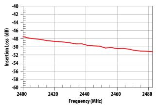
Figure 11. Tx–Ant Rejection in Bluetooth Band.
