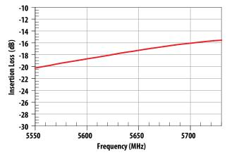
Figure 14. Tx–Ant Rejection at Tx Third Harmonic.
