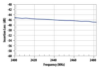
Figure 12. Ant-Rx Rejection in Bluetooth Band.
