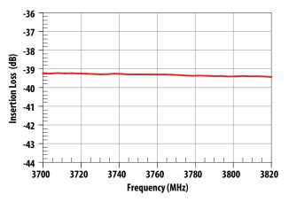
Figure 13. Tx–Ant Rejection at Tx Second Harmonic.
