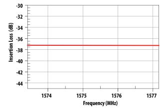
Figure 8. Tx-Ant Rejection in GPS Band.
