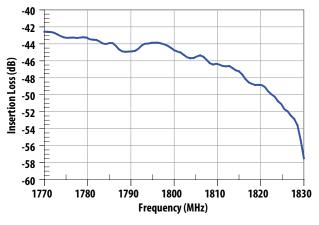
Figure 15. Ant–Rx Rejection, 1770–1830 MHz.
