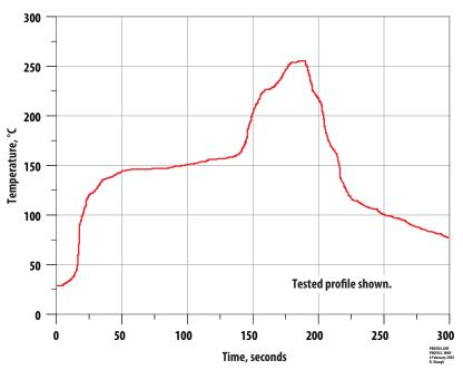
Figure 33. Verified SMT Solder Profile.
