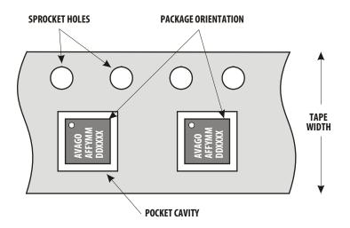
Figure 31. Unit Orientation in SMT Tape.
